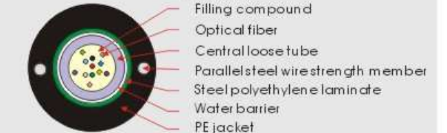
Outdoor Armoured Loose Tube Cable(2-12F) GYXTW
